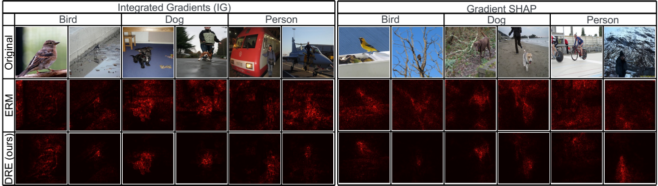
Figure 3. Integrated Gradients (IG) [17] and Gradient SHAP [10] saliency maps for out-of-distribution data from VLCS [4] dataset. Using VOC2007 [3] as the testing set, for ERM model the saliency maps of both Integrated Gradients (IG) [17] and Gradient SHAP [10] methods are excessively focused on background pixels, such as branch and ground. Our explanations significantly alleviate the salience of spurious correlations and clearly depict the contour of the object.
