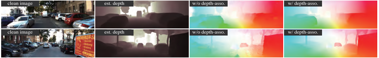
Figure 2. Effectiveness of depth association. Depth contains rich structure information, facilitating the optical flow rigid boundaries sharp.
