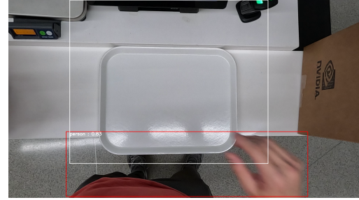
Figure 3. Three white lines define our RoI. The one on the left is called left_vertical , one on right is called right_vertical and the one which is horizontal is called lower_horizontal
