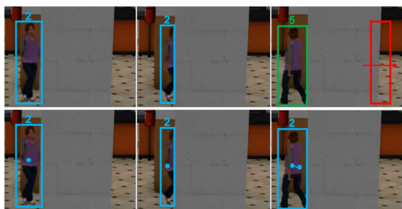
Figure 5. In the first row, an incorrect local ID was assigned as a result of calculating the IoU ratio with the bounding box predicted by the Kalman filter. The red box indicates the bounding box that is predicted by Kalman filter. In the second row, the correct ID was assigned by using the Euclidean distance between the bounding boxes detected at the previous time step and the current time step.
