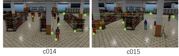
Figure 4. Example of matching points annotation between 2 cameras
