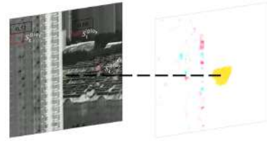
Figure 6. Schematic diagram of the matching between the optical flow map and the detection results of YOLOv7, where S_t^{glo2} is the closest to l_t^{of} , yet S_t^{glo2} does not contain the target.
