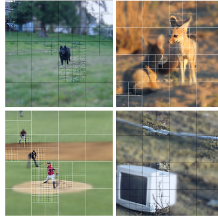
Figure 2. Tokenizations obtained using our saliency-based Quadtree. For clearer visualization, we upsample patches back to their original size after the tokenizer resizes them to a fixed representation size. Notice how high-saliency regions are represented in high resolution while background regions are blurry.
