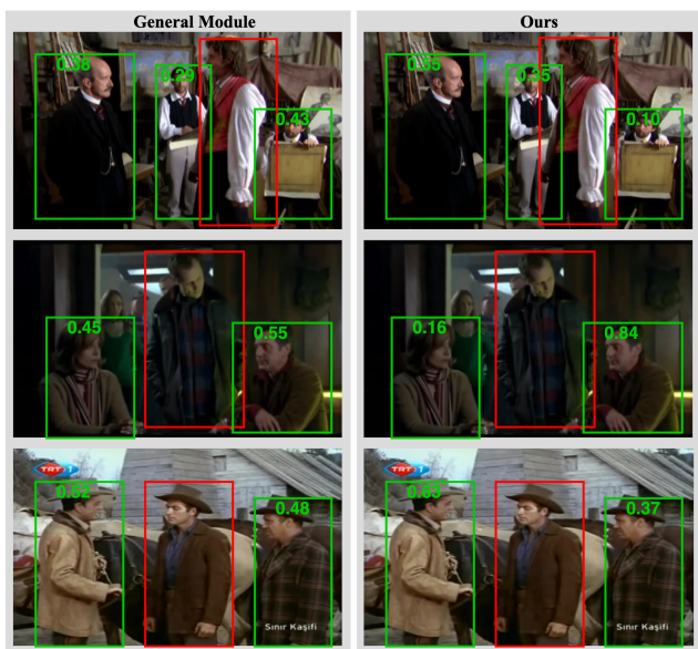
Figure 4: We visualize attention weights from our TransPC and the general person-person interaction module. The actors of interest are in the red boxes and the other actors are in the green boxes. In each image, we remove the weight of actor of interest and re-normalize the rest attention weights to 1.
