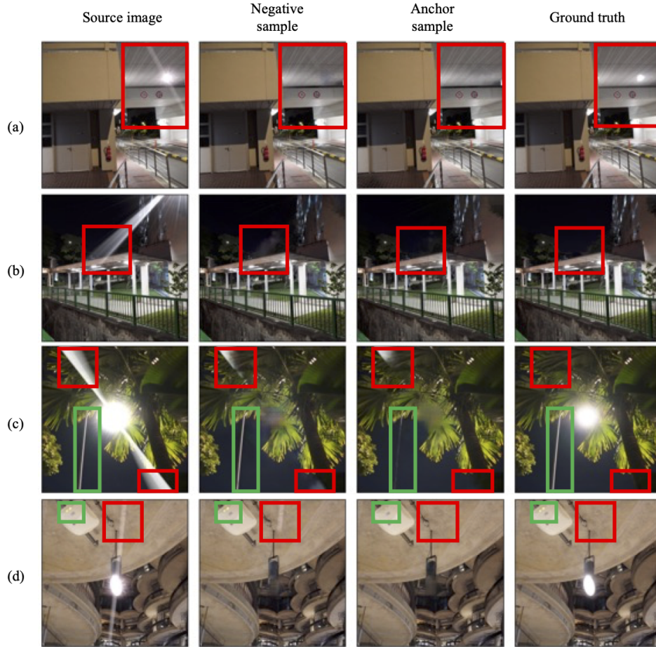
Figure 3. Comparing the two output samples from negative(reference) and anchor(proposed) networks: quantitative results of the negative and the anchor samples in terms of PSNR and SSIM (negative/anchor) for synthetic flare dataset: (a) 29.40 / 30.12, 0.9895 / 0.9883 (b) 33.88 / 34.37, 0.9598 / 0.9689 (c) 17.44 / 16.66, 0.9058 / 0.9000 (d) 22.37 / 21.94, 0.9731 / 0.9751
