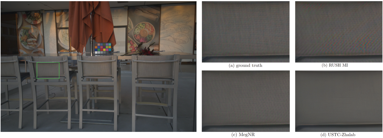
Figure 5. Qualitative image quality (IQ) comparison. The results of one of the test scenes (42dB) are shown. Detail loss or false color in the top three methods in Table 1 can be found when compared with the ground truth. The mesh of the chair is over-smoothed to different extents in (c) and (d) and some false color can be found in (b). The RGB images are obtained by using the ISP in Fig. 2, and its code is provided to participants.
