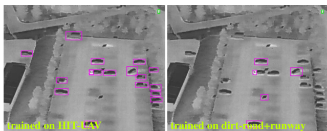
Figure 6. Qualitative results showing the performances of Faster R-CNN in a scene from HIT-UAV with different training datasets.
