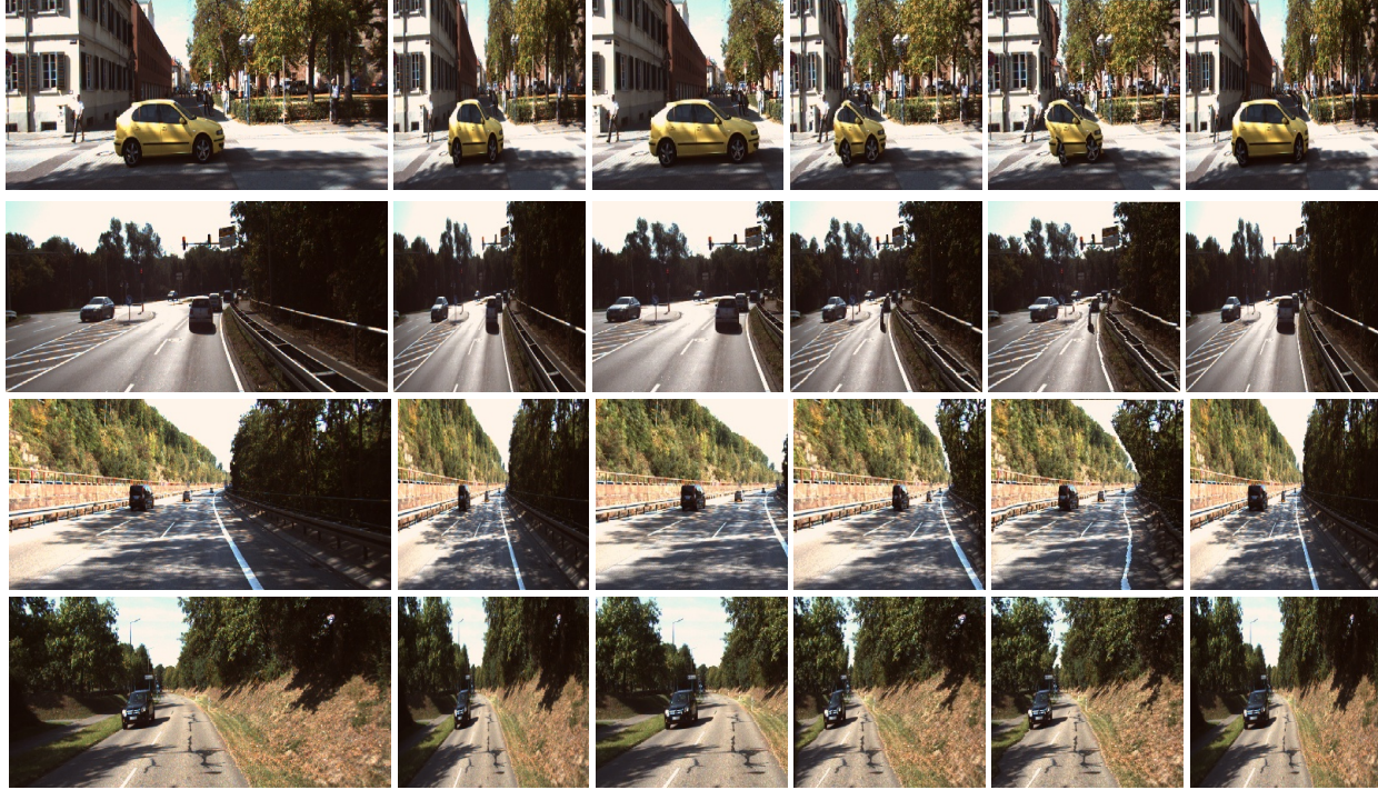
Figure 6. Qualitative results of stereo video retargeting on randomly selected left video frames from the KITTI stereo 2015 [21] (top) and 2012 [10] (bottom) datasets for reducing the horizontal video size at 50%. Left to right: original frame, linear scaling, manual cropping, seam curve [1], fast video [4], and ours.
