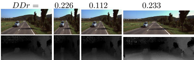
Figure 8. Different retargeting results with respective depth maps. Left to right: Input video frame and their retargeted results with horizontal size reduction at 50%, 20%, and 15% (enlarge).
