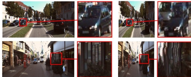
Figure 10. Example of failure cases due to: (top) videos with many salient objects and (bottom) wrong detection of salient objects.
