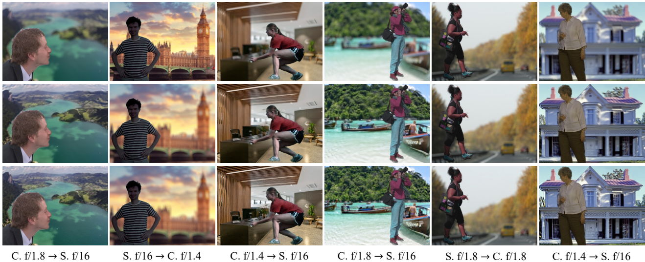
Figure 9. Visual results of our method and Restormer [72] on the Bokeh effect transformation task. Top row shows the input images and second row shows the Restormer’s results. Last row shows the transformed results generated by our method. In addition, lens transform information is shown in the bottom. ‘S. f/1.8 → C. f/16’ means the image is transformed from Sony50mmf1.8BS to Canon50mmf16.0BS .
