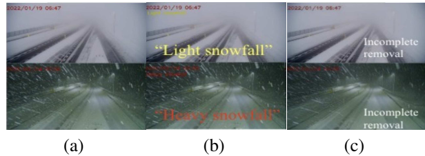
Figure 5. Comparison of snowfall detection in real images: (a) original image. (b) “Light snowfall” and “Heavy snowfall” by DeepSnow. (c) Failure cases by Transweather.
