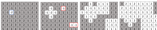
Figure 2. At t_n \leq -2 , a connected component is born, and at t_n \leq -1 , two other connected components are born. When t_n \leq 1 , the upper component with birth-time -1 is killed and merged into the one with birth-time -2 . Finally, when t_n \leq 2 , the right component with birth-time -1 is killed. As a result, the 0-th barcodes of the dataset can be computed and represented as [-2, \infty) , [-1, 1) , and [-1, 2) . This barcode representation provides a concise and informative summary of the topological structure of the dataset. Image is from [23].
