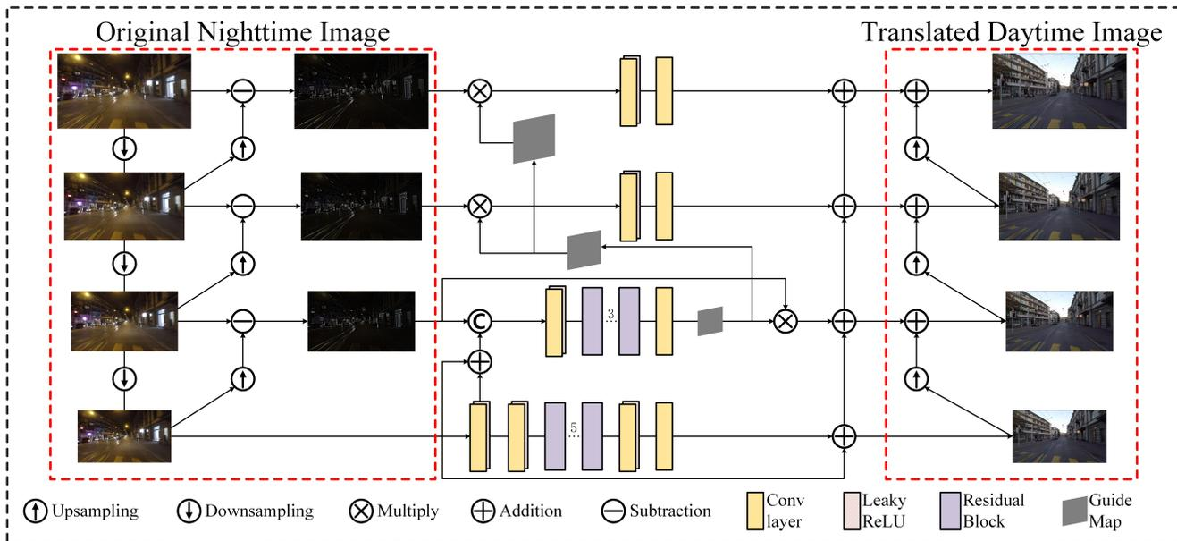
Figure 2. The framework of our developed N2D-LPNet for nighttime driving scenes. The red boxes are the input and output streams of the pyramid network. We make full use of inter-frequency priors which utilize each lower frequency information to refine the higher frequency feature in a progressive manner.
