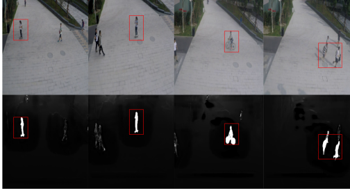
Figure 8. Qualitative results for the motion branch. Top: Input frames. Bottom: Anomaly maps. Anomalies are indicated by red bounding boxes.
