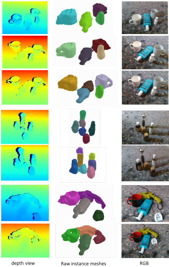
Figure 8: Qualitative results on real scenes with non-convex objects. The raw mesh segmentation of SIMstack is able to estimate shape and decomposition of scenes with non-convex objects.
