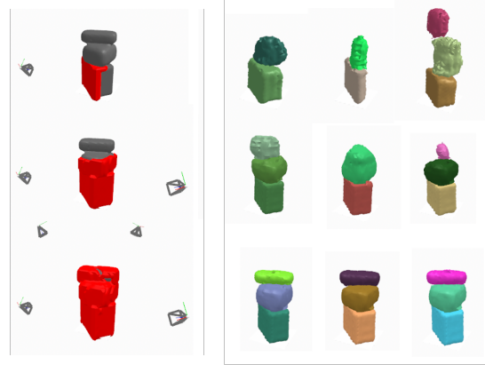
Figure 10: How sampling variety changes as views are added. Left: Ground truth and visible mesh area overlay (red). Right: 3 random latent space samples (without SQ fitting) for each view; as data is added the samples are increasingly constrained.
