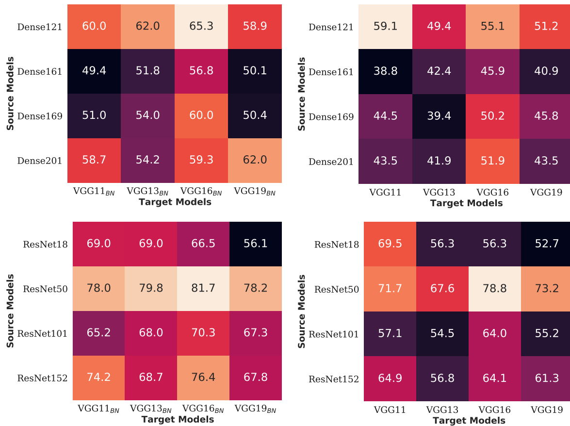
Figure 2: Batchnorm Vulnerability to Targeted Transferability : {10-Targets (all source) settings}. TTP (Algorithm 1 in the paper) strength is higher against models trained naturally with batchnorm as compared to without batchnorm. Batchnorm [8] provides better optimization and increase model clean accuracy but these empirical results indicate that it also make the model more vulnerable to blackbox targeted attacks. Each value is averaged across 10 targets (see Section 4 in the paper for details) with 49.95k ImageNet val. samples for each target. Perturbation budget is l_\infty = 16 .
