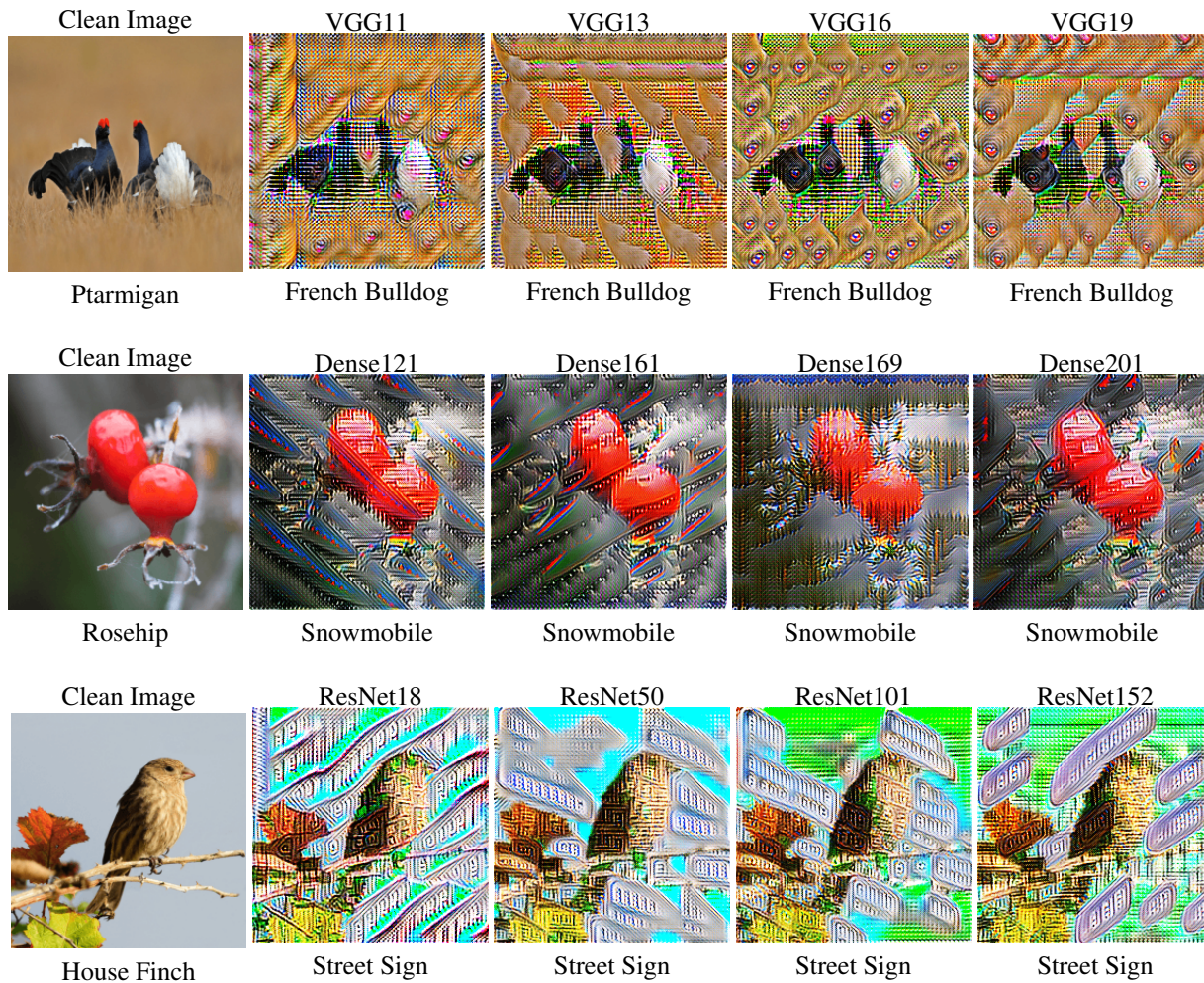
Figure 9: Evolution of TTP: Unconstrained targeted adversarial patterns generated by TTP are shown to demonstrate how TTP evolves as it learns perturbations from different source models of a certain family of networks.
