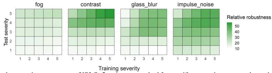
Figure 12. Relative robustness improvement on YOLOv5s using our method for specific corruption types and severity levels on Pascal-C.
