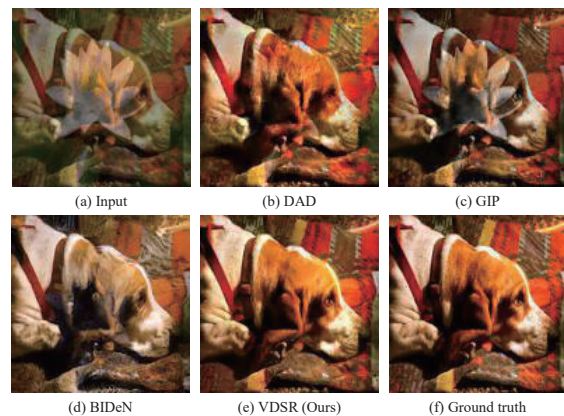
Figure 1. Image decomposition results on the Stanford-Dogs [23] + VGG-Flowers [29] dataset. We only present one output here. It can be observed that both DAD [51] and GIP [52] contain blurred edges of “flower”, and BIdeN [14] produces slight blur and color distortion. Our result preserve finer geometric structures.
