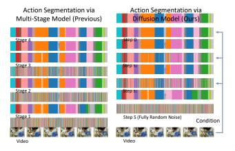
Figure 1. **Multi-stage model vs. diffusion model for action segmentation.** They both follow an iterative refinement paradigm. *Left*: Many previous methods utilize a multi-stage framework to refine the initial prediction. *Right*: We formulate action segmentation as a frame-wise action sequence generation problem and obtain the refined prediction by an iterative denoising process. Colors in the barcodes represent different actions.
