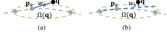
Figure 4: Visual illustration of the difference between (a) P2P and (b) P2T distances when \Omega(\mathbf{q}) is sparse. We also refer readers to Table 5 for the quantitative comparisons.
