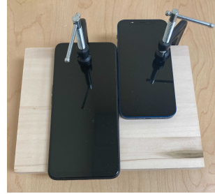
Figure D.3. Set up to test the accuracy of the gyroscope. Rig to ensure identical rotations between the two phones to assess the accuracy of the ground truth of the BUSS dataset.
