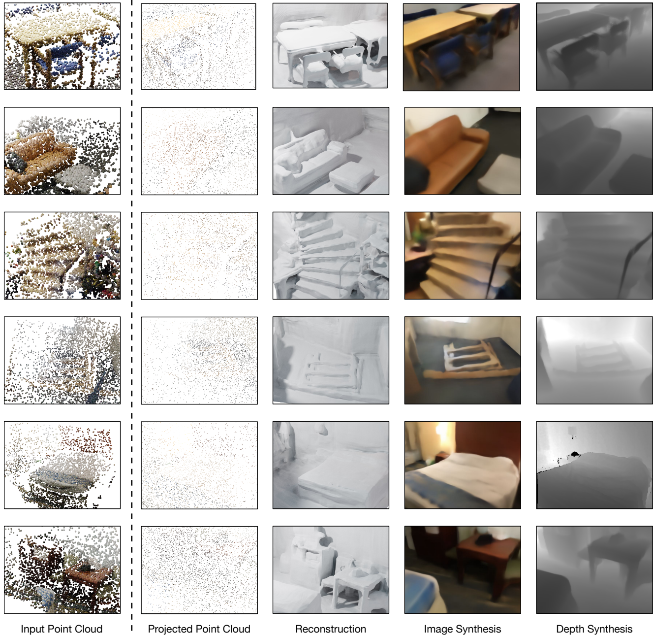
Figure 4. More results of application examples of Ponder on the ScanNet validation set (part 1). The input point clouds are represented by large spheres for improved clarity. The projected point clouds illustrate the actual sparsity of the point data.
