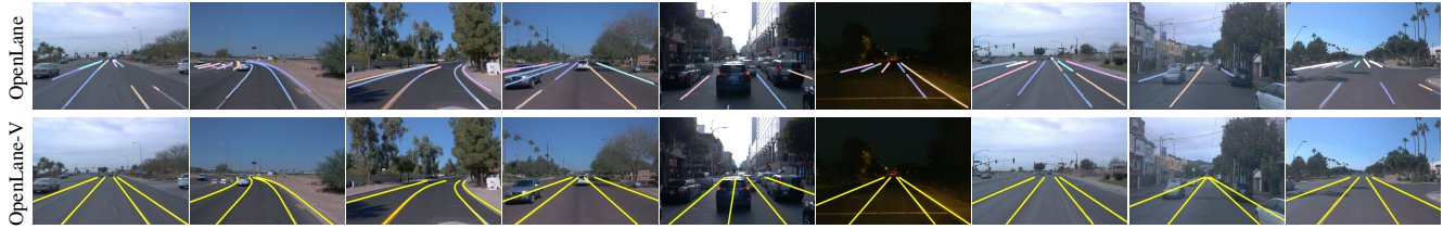
Figure 6. In OpenLane, only visible lane parts are annotated, so the same lane may be split into multiple parts. In contrast, in OpenLane-V, each lane is seamlessly annotated, depicted by a yellow line, and invisible parts are inpainted.
