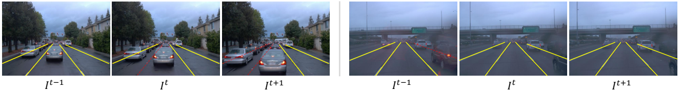
Figure 4. In OpenLane, totally invisible lanes are not annotated. They cause flickering artifacts as depicted by dotted red lines. To overcome this issue, we manually annotate such lanes using the information in adjacent frames.
