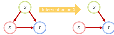
Figure 5: An example of the causal graph and causal intervention. We study the causal relation X \rightarrow Y while confounder Z exists and brings bias. After the intervention on variable X , the poisonous relation Z \rightarrow X is eliminated.
