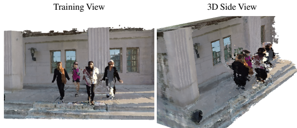
Figure 4: 3D samples. Erroneous geometry reconstruction at regions invisible during training harms 3D clustering quality.
