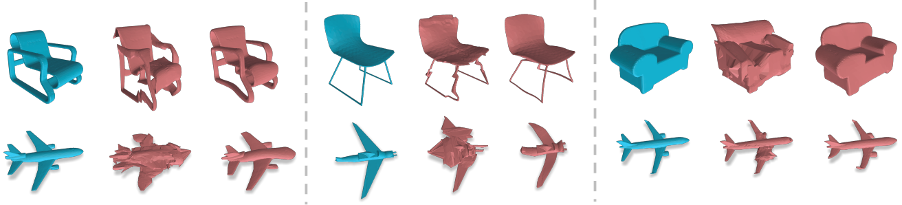
Figure 1. The effectiveness of the mesh smooth layer. For every three shapes, the leftmost one is the reference shape for deformation, the middle one is the generated mesh without smoothing, and the right one is the shape after smoothing.
