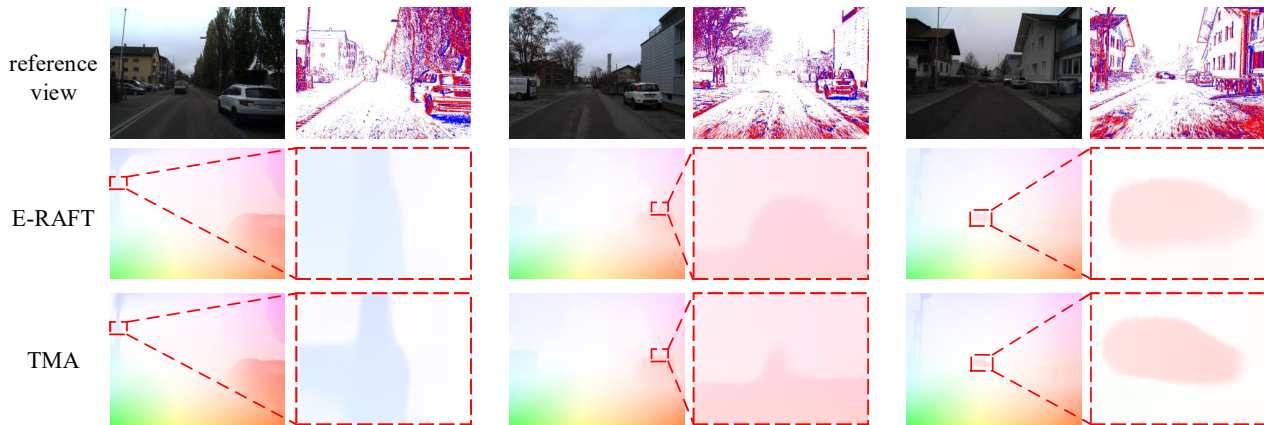
Figure 1: More qualitative results on DSEC-Flow. For each two columns, we show the reference image and event frame and compare our method with the state-of-the-art E-RAFT [2]. Significant improvements are highlighted by red boxes.
