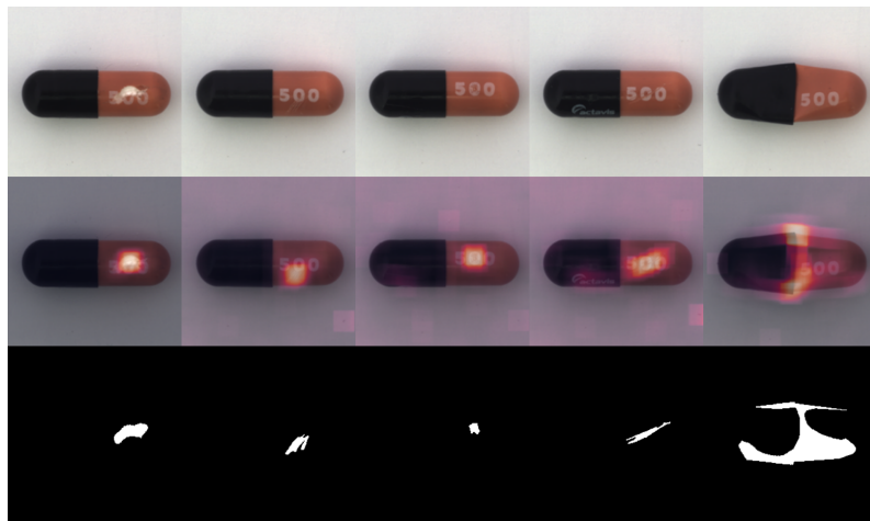
Figure 8. Anomaly localization examples of the capsule category. From top to bottom: input image, restoration error map, ground truth.
