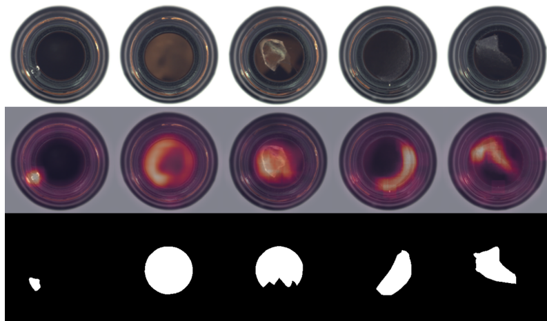
Figure 6. Anomaly localization examples of the bottle category. From top to bottom: input image, restoration error map, ground truth.
