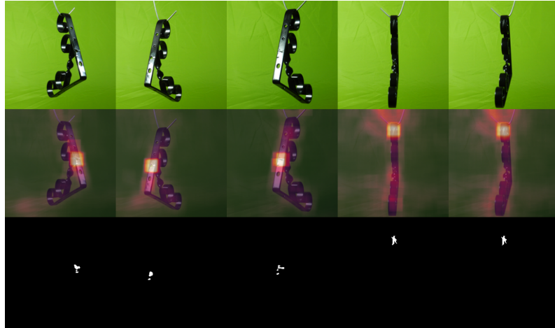
Figure 19. Anomaly localization examples of the bracket black category. From top to bottom: input image, restoration error map, ground truth.
