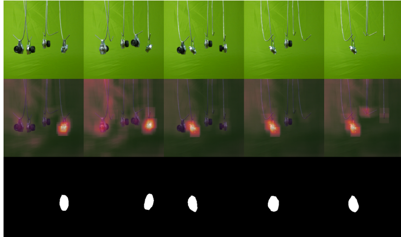
Figure 22. Anomaly localization examples of the connector category. From top to bottom: input image, restoration error map, ground truth.
