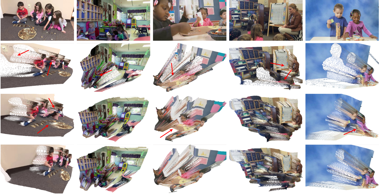
Figure 1. Comparison of point clouds generated using the depth maps from Ranftl et al. [15] (row 2), Wei et al. [18] (row 3) and Patakin et al. [14] (row 4) on ChildPlay images. The point clouds generated using Patakin et al. appear to best preserve the geometry of the scene.
