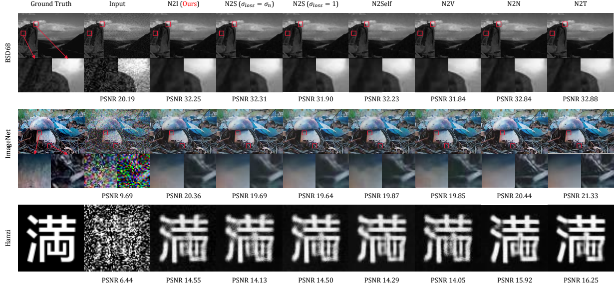
Figure 5: Result demonstration without cherry-picking. We display outputs of methods including N2I , two versions of Noise2Same , Noise2Self , Noise2Void , Noise2Noise , and Noise2True with their PSNRs of 3 figures from 3 datasets.
