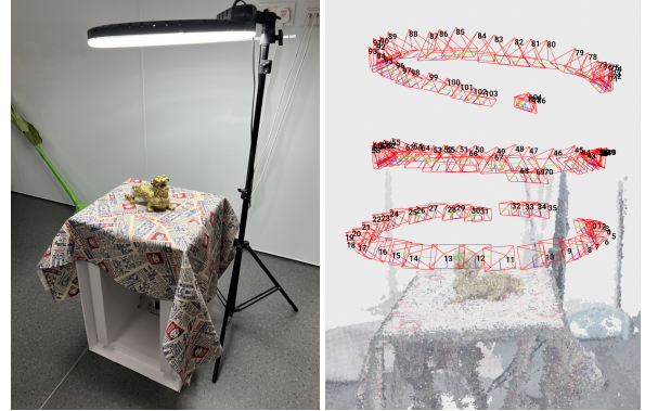
Figure 3. Capturing setup for the NeILF-HDR dataset. The left image shows the lighting setup, and the right image illustrates the camera trajectories.
