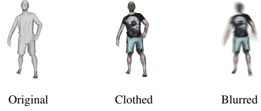
Figure E.1. BC-CAPE dataset construction. The original CAPE [9] human body dataset contains no texture or clothes. Since their human body representation is also an SMPL [12] model, we use textures from the SURREAL [16] dataset. Then, blurry inputs are generated by temporal integration and interpolation between neighboring recorded meshes.
