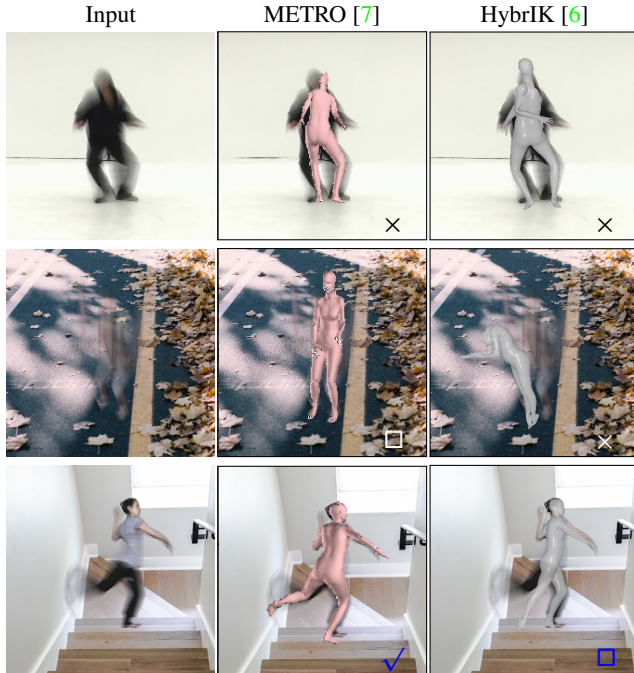
Figure E.3. Failure of initial human pose estimation. In some cases, when the initialization is far from the real pose, our method cannot converge to the right solution. We have notations for three cases: (✓) converges and initial pose is one of the sub-frame poses, (□) still converges but initial pose is not one of the sub-frame poses, and (×) does not converge. In the top row, both models predict a flipped pose, which optimization cannot rotate back. The middle row shows a fast squatting pose with stretched arms, for which only the METRO [7] initialization allows for convergence by predicting a standing pose. In the bottom row, only the METRO [7] detects the moving leg.
