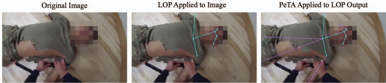
Figure 5. An example of the application of our Pose-Enhancing Transformation Algorithm (PeTA). From left to right, this figure shows the input image, the image following the application of the Lightweight OpenPose (LOP) [21] algorithm, and finally the image after using PeTA to infer the missing joints. Note that the face is blurred for the purposes of this paper, but is not blurred for LOP or PeTA algorithms.
