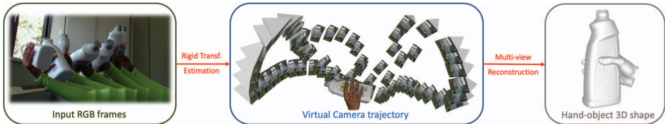
Figure 2: Hand-Object 2-stage 3D reconstruction pipeline. Given an RGB video of a hand holding an object (left), the rigid transformation between frames is first estimated. This allows to see the problem as if a set of multiple virtual cameras observe a fixed hand-object system (middle). Multi-view reconstruction can then be employed to estimate an accurate hand-object 3D shape (right). We benchmark several baselines for both stages using the presented dataset.
