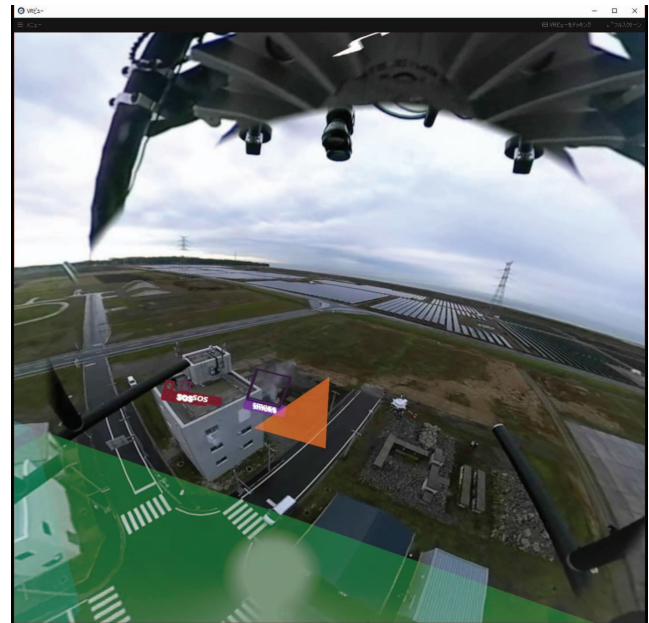
Figure 4. Situation presentation by VR. The results detected as "call for help" are shown as "SOS" in red BBOXes. The detected smoke is highlighted with a purple BBOX.
