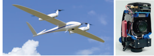
Figure 2: Vertical take-off and landing drone (left) with integrated camera system MACS-Micro (right).
