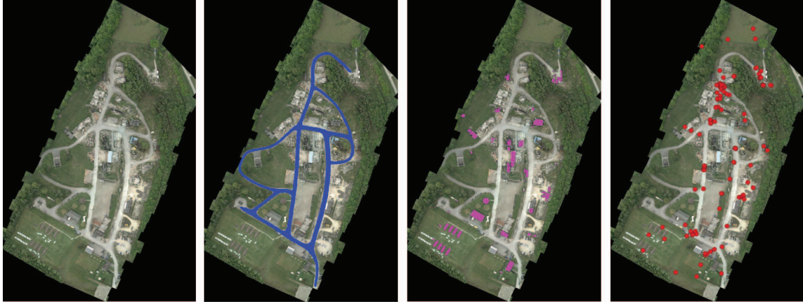
Figure 5: Qualitative results: image mosaic, segmented roads, segmented buildings, and detected people (left to right).
