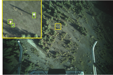
Figure 4: View from the delivery drone and demonstration of the onboard person detection algorithm.
