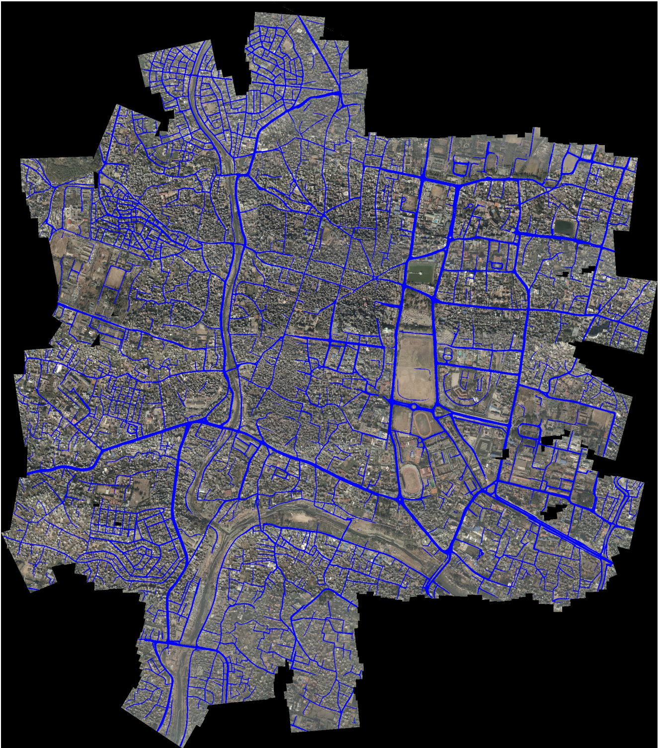
Figure 9: Road segmentation results for a scene from Kathmandu in Nepal captured from a UAV at 8 cm/px and resampled to 50 cm/px.
