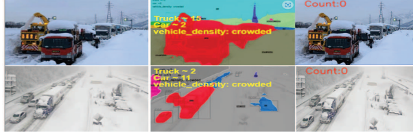
Figure 9. Object counting results in images with traffic jams. (1) Winter traffic jam images. (2) Proposed Dcount. (3) SOTA: CLTR[40].
