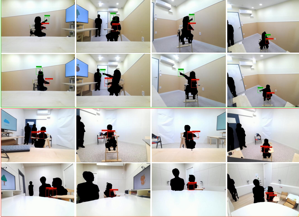
Figure 5. Examples of result images on the ASD-Pointing dataset. The green and red colors represent test cases where pointing is performed and not performed, respectively. The videos were captured with four Azure Kinect cameras in three living lab spaces.
