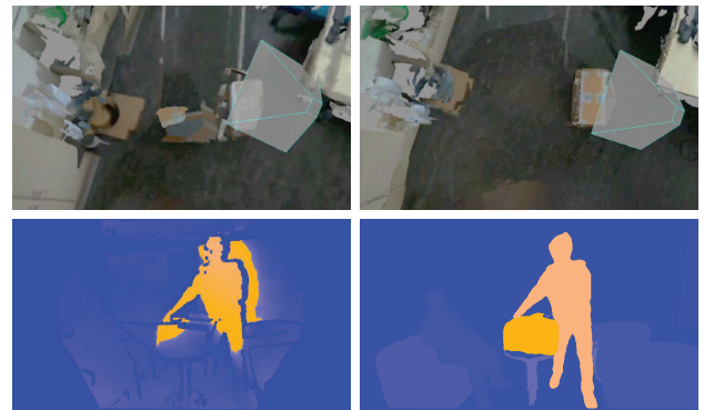
Figure 4: Comparison of design choices of the proposed pipeline. Top row: An example output from the exploration client using the standard voxel block weighting schema (left) vs. exponential weight decay via weight capping. The second approach yields a reconstruction of the box with fewer artifacts. Bottom row: Thresholding of the normalized EPE before (left) and after (right) propagation of the error modes into the static (blue) and dynamic (yellow) object masks. Again, the second approach produces a more plausible segmentation into static and dynamic regions.
