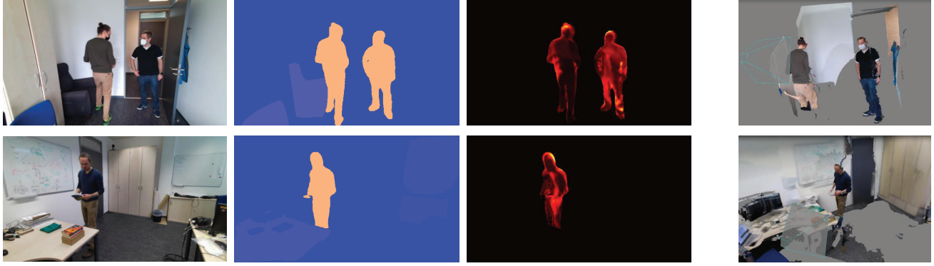
Figure 3: Results of our approach on different scenes. Left to right: Input color image; resulting segmentation into static (blue) and dynamic (yellow) regions; the accumulated 3D flow magnitude; a novel view of the scene as visualized in the exploration client.
