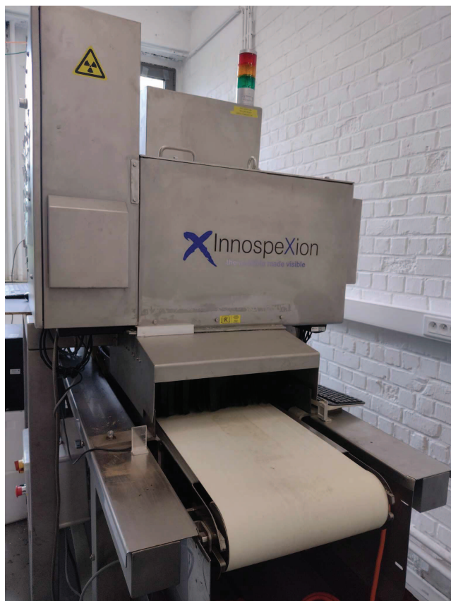
Figure 1. Prototype industrial line scanner with conveyor belt (InnospeXion), available in the lab. Device used for collecting X-ray imaging datasets.
