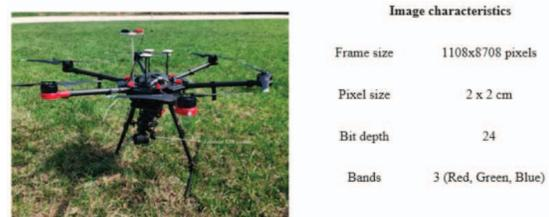
Figure 2: The UAV DJI M600 hexacopter platform used for image collection, equipped with a phase one IXU 1000 RGB camera and some characteristics of the image.
