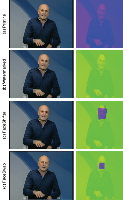
Figure 5: Example of input/output pairs from the detector. The model was trained using \alpha = 0.002 and SSIM as reconstruction loss. The output is green in regions where the watermark was detected, and blue where it was not. Similar results obtained with models trained with MSE are given in Appendix B.
