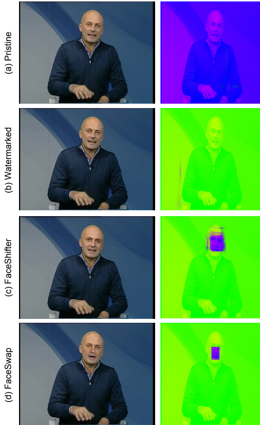
Figure 10: Example of input/output pairs from the detector. The model was trained using \alpha = 0.002 and MSE as reconstruction loss. The output is green in regions where the watermark was detected and blue where it was not.
