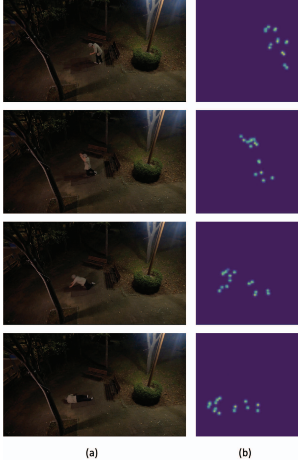
Figure 2: Examples of generated heatmaps through the frames. (a) is the RGB frame, while (b) is the generated pseudo joint heatmap.
