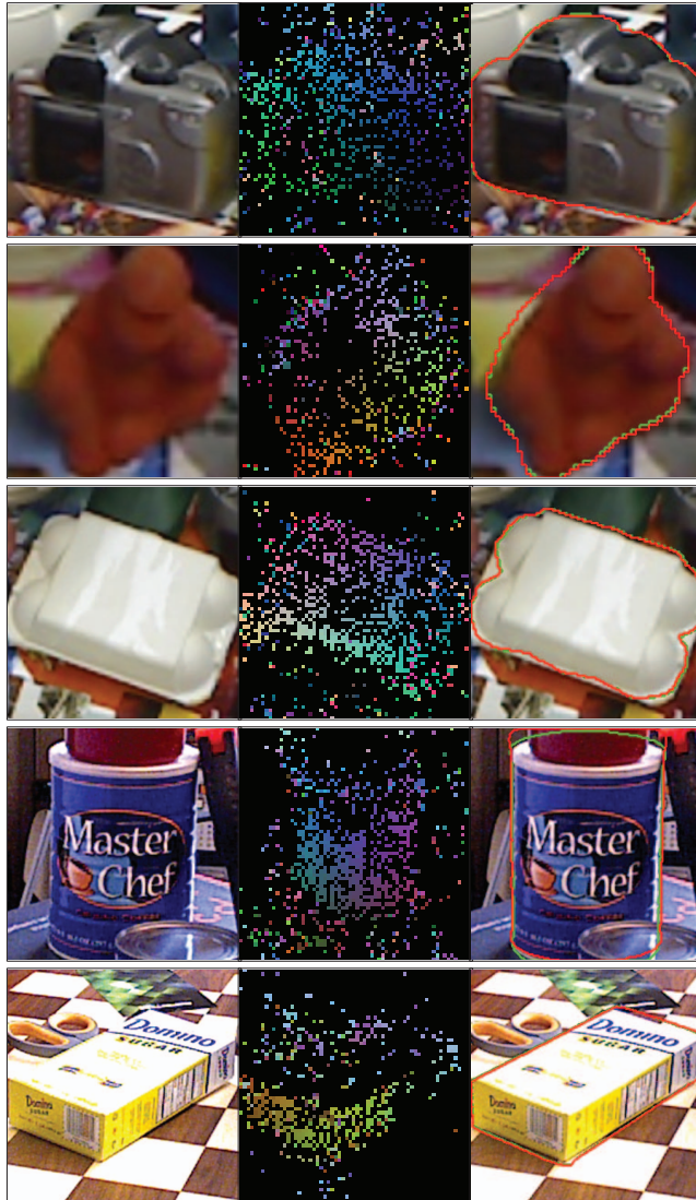
Figure 6: Visualization of matching keypoints. Here we show PoseMatcher output \mathcal{C} , where we assigned a normalized coordinate of the highest confidence keypoint to the corresponding pixel. The last two rows are examples from the YCB-V dataset.
