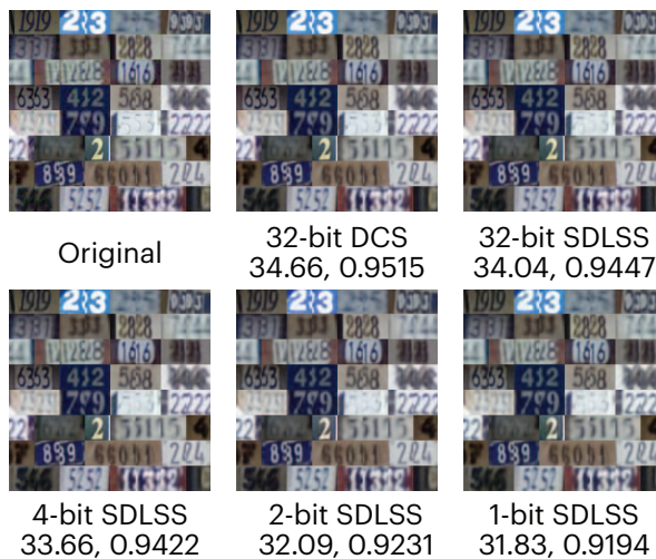
Figure 5. SVHN images reconstructed using Q-GEN models and 32-bit DCS model are compared here. We observe comparable visual performance from low-precision Q-GEN models compared to full-precision models.
